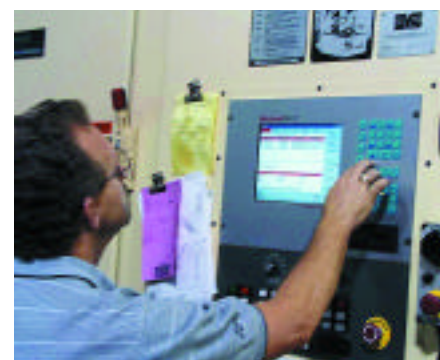
Attached to a Sunstrand five-axis Omnimill with rotary table and pallet changers, the MachineMate MM5 control could control 8 axes simultaneously if it had to. Power and multi-axis capability is no longer an issue
